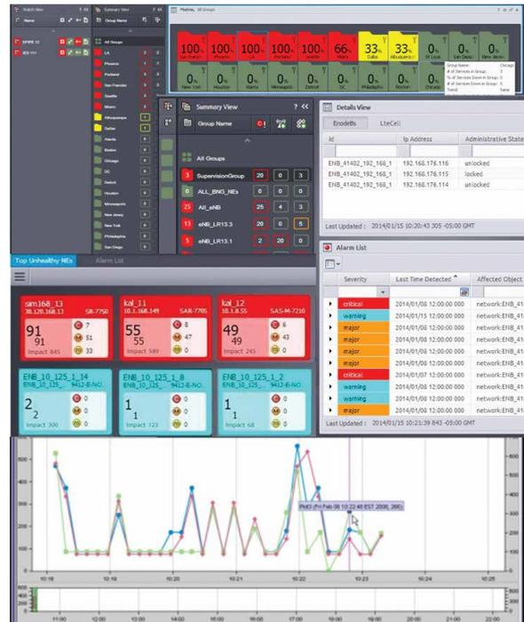
OAM test suites can be scheduled and compared to configurable parameters – such as jitter, delay and packet-loss metrics – to proactively detect network and service degradation. Rules-based alarm notifications, such as threshold-crossing alerts and escalating test failure alerts, further automate assurance and adherence to performance and QoS objectives.
